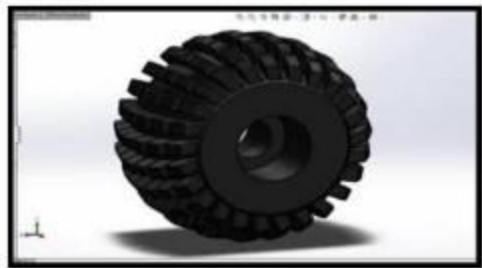
Fig 2: Wheels Wheel is simple and mad from hard fiber and plastic only. The wheels are needed to be wider for increasing the traction to traverse upon the obstacles. And their diameter depend upon the availability and amount of speed required. The actual rover uses billet wheels, and machine the wheel and tread from one piece of round aluminum stock.
